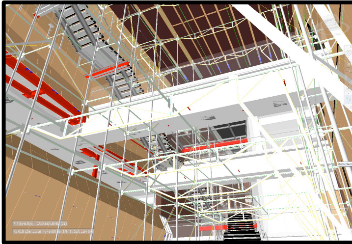
Figure 2: View of Atrium During Stair C and Screen Wall Installation
